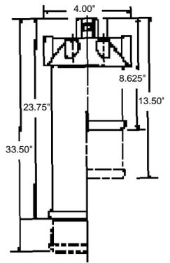
Allow a minimum of 2 1/2" clearance for cartridge change
